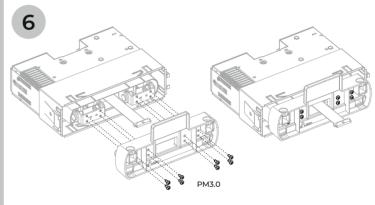
Put the radio main unit and monitor stand together
