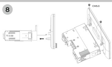
Install the radio main unit and fix the display
