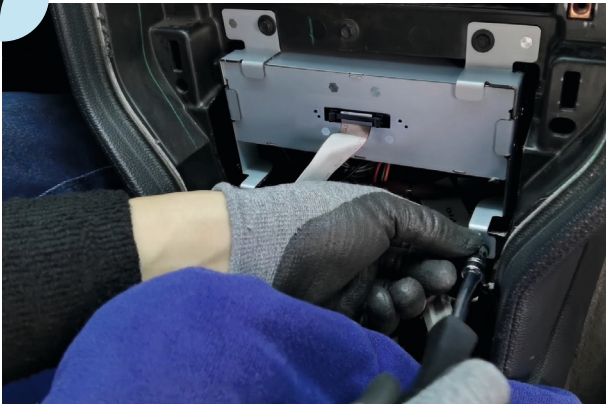
Dynavin main unit installation
