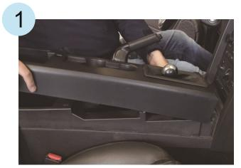
Remove the screws and pry up the armrest box
