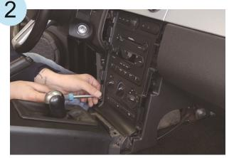
Remove the left and right side panels and remove the screws
