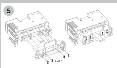
Put the radio main unit and monitor stand together
