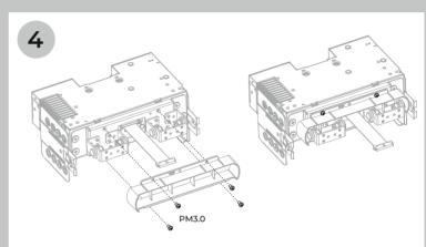
Put the main unit and rotary damper together
