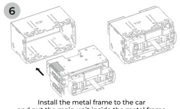
and put the main unit inside the metal frame
