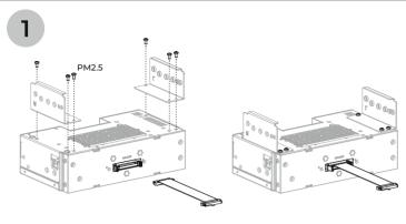
Put the main unit and metal bracket together and connect the connection cable to the main unit
