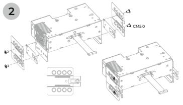
Put the main unit and mounting plates together
