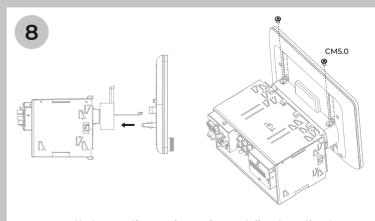
Install the radio main unit and fix the display
