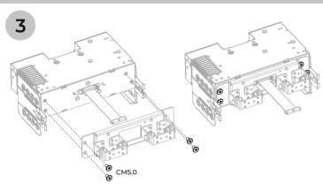
Put the main unit and rotary damper together
