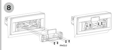
Put the radio main unit and monitor stand together
