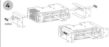
Put the main unit and rotary damper together Put the main unit and mounting plates together
