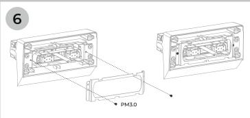
Put the main unit and the metal plate together
