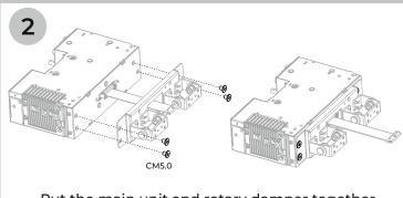
Put the main unit and rotary damper together
