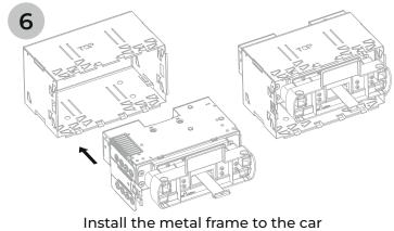
Install the metal frame to the car and put the main unit inside the metal frame
