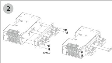
Put the main unit and rotary damper together
