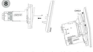
Install the radio main unit and fix the display
